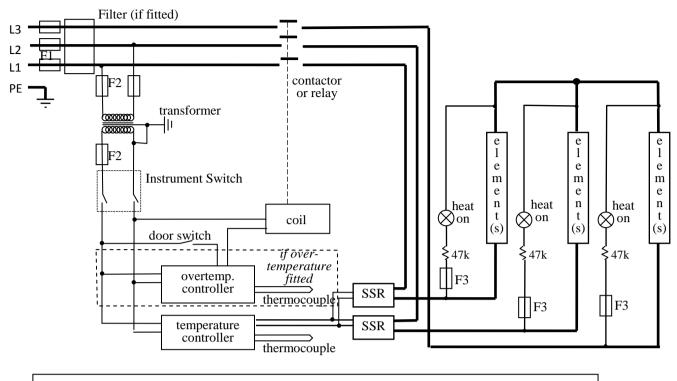
In this configuration the fuses F2 on the supply side of the transformer may be GEC Safeclip, not 32 x 6mm glass as stated in section 8.0.
